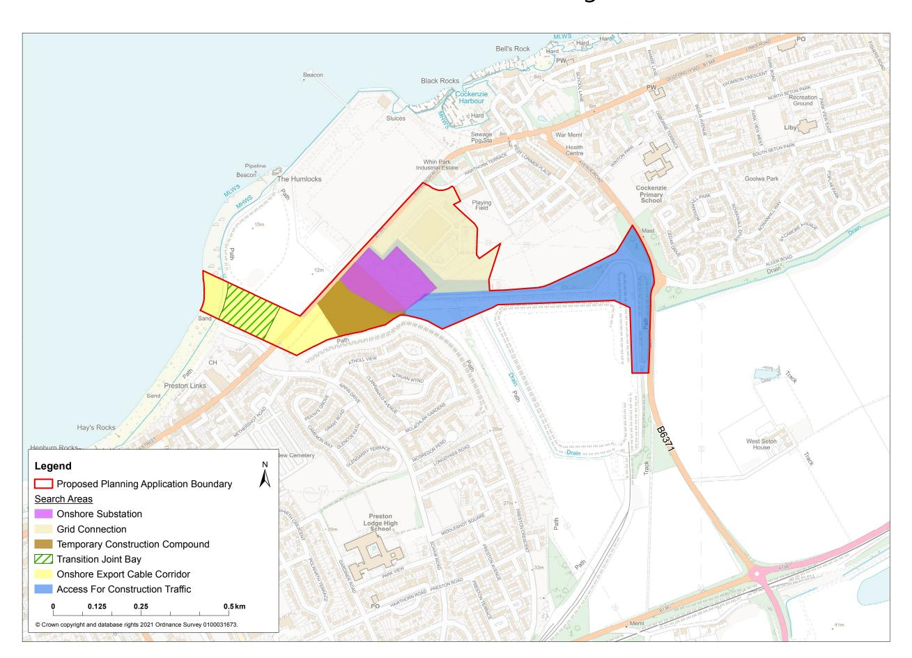
At landfall and under the B1348 Edinburgh Road, it is anticipated that the onshore export cable will be installed using a form of directional drill or other trenchless techniques to minimise potential impact to users of the beach and the B1348 respectively. The remainder of the onshore export cable will be installed using open cut trenching. Once installation of the cable is complete, the land will be fully reinstated and restored.
